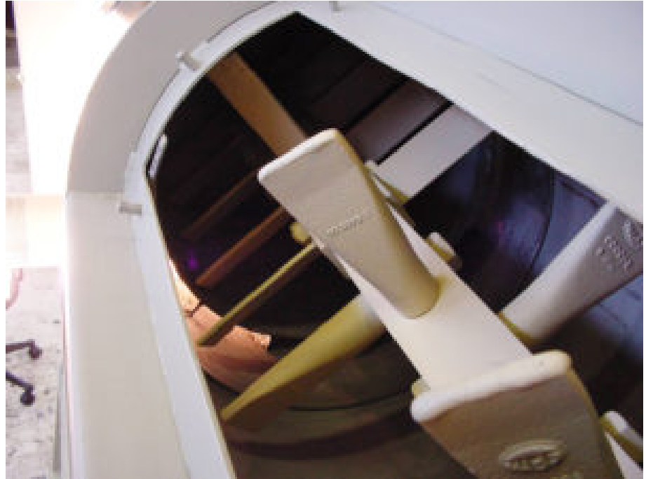
Preconditioner mixing zone. Photo courtesy of California Pellet Mill.
