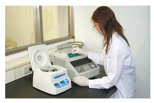
While useful for several types of tests, polymerase chain reaction requires the use of an expensive programmable thermal cycler (right).
