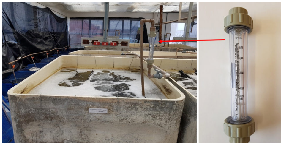
Left: View of experimental unit with coupled rotameter (right); rotameter used to control aeration intensity (left).
