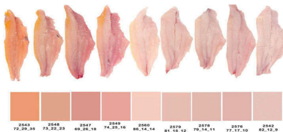
Fig. 1: Photos of catfish fillets taken by a Canon 40D digital camera in the light box with set configurations and corresponding average colors of the whole fillets after blurred in Adobe Photoshop. The readings below the color cubes were formatted as identification number and CIELAB values.
