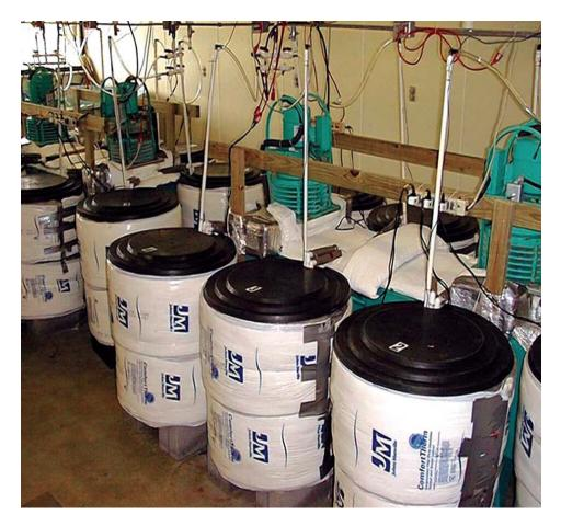
The system was initially developed with four individual unit chillers in two central tanks.
