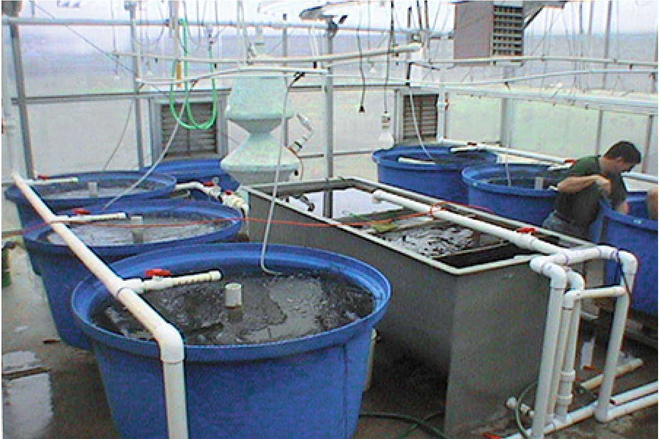
Fig. 1: Water from the six 540-l polyvinyl tanks drained into a manifold that emptied into a settling tank.
