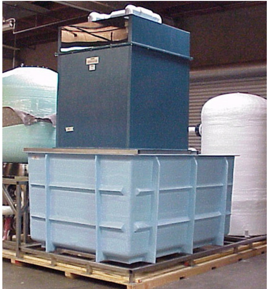
Large trickle filter. Photo courtesy of Aquanetics Systems, Inc.
