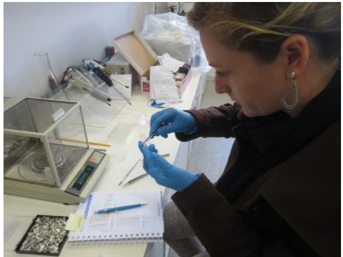
Weighing samples for stable isotopes analysis.
