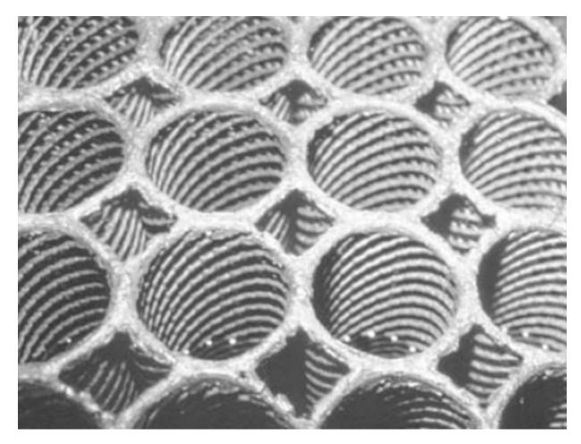
The biofilm established in the Bioblocks improves sedimentation by attracting small particles.
