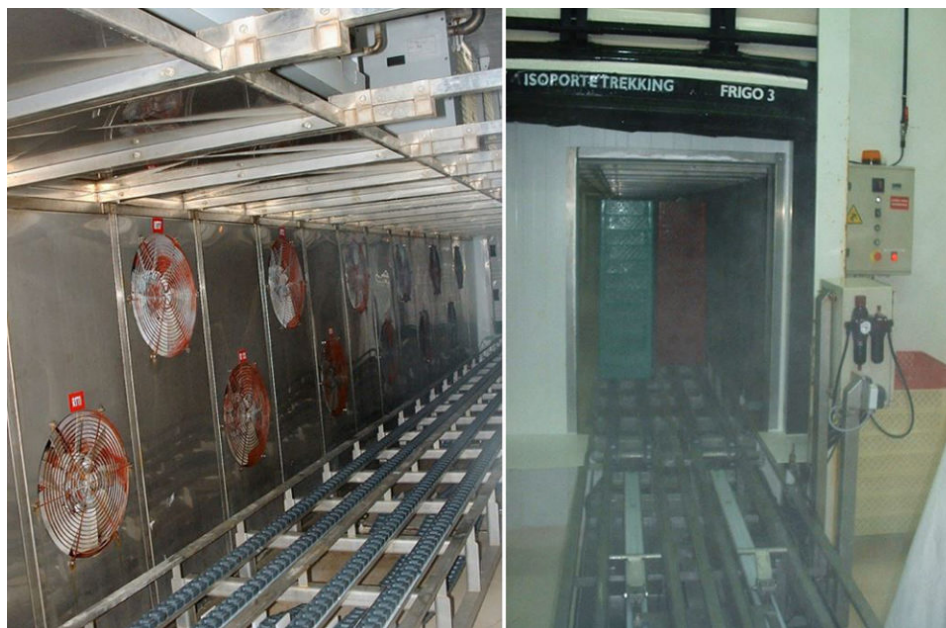
Views of air blast tunnel: inside an air blast tunnel (left); and piles of shrimp blocks going into the tunnel (right).
