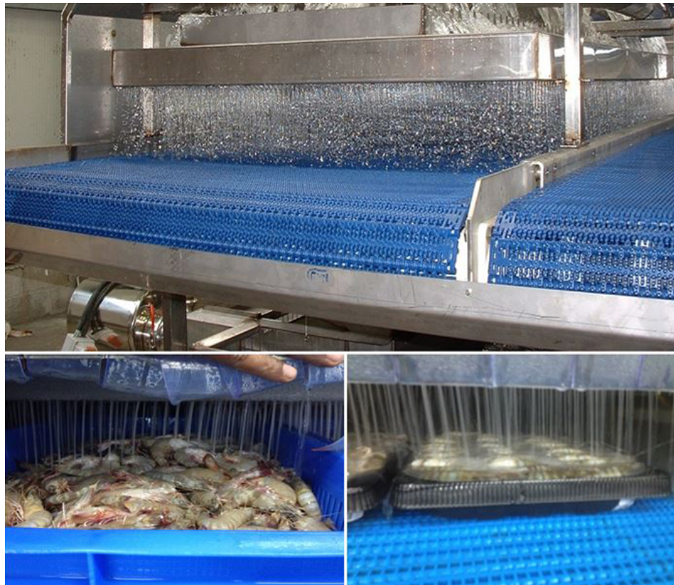
Views of a brine freezer (top); and shrimp being frozen by shower of brine (bottom).
