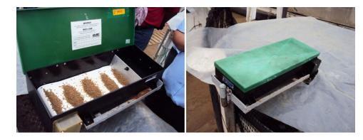
Shrimp are constantly feeding or grazing, so continuous feeding using belt feeders such as this one is a recommended practice.
