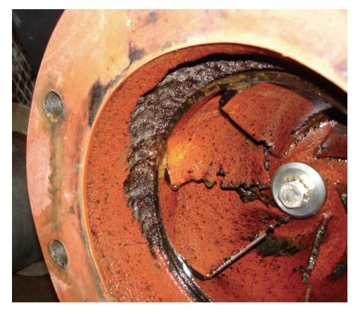
The destructive effects of cavitation can become evident after only several months of pump operation.
