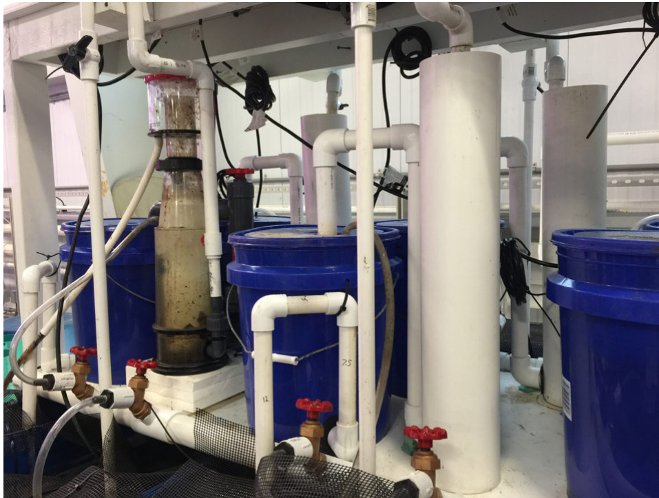
Filtration components such as foam fractionators and external biofilters may be used for RAS nursery production.
