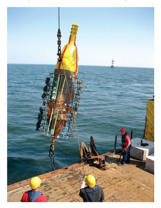
One element of the MytiFit project involves an evaluation of blue mussel attachment to varied artificial substrates that could be used for culture at offshore wind farms.
