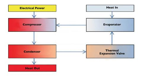
Fig. 1: Basic refrigerant flow.
