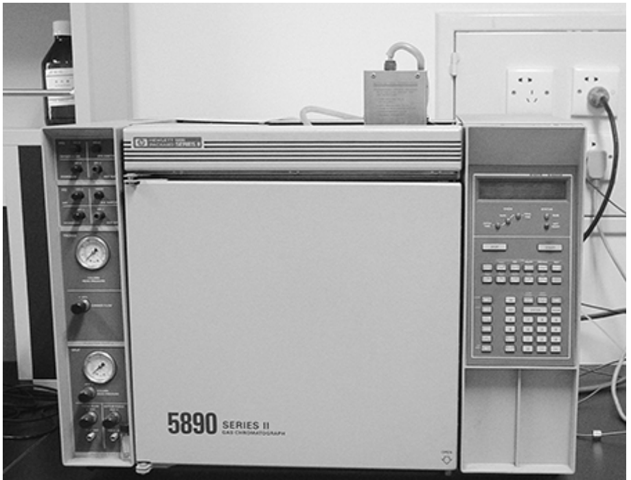
Gas chromatographers are used for separation, identification and quantification of volatile compounds.
