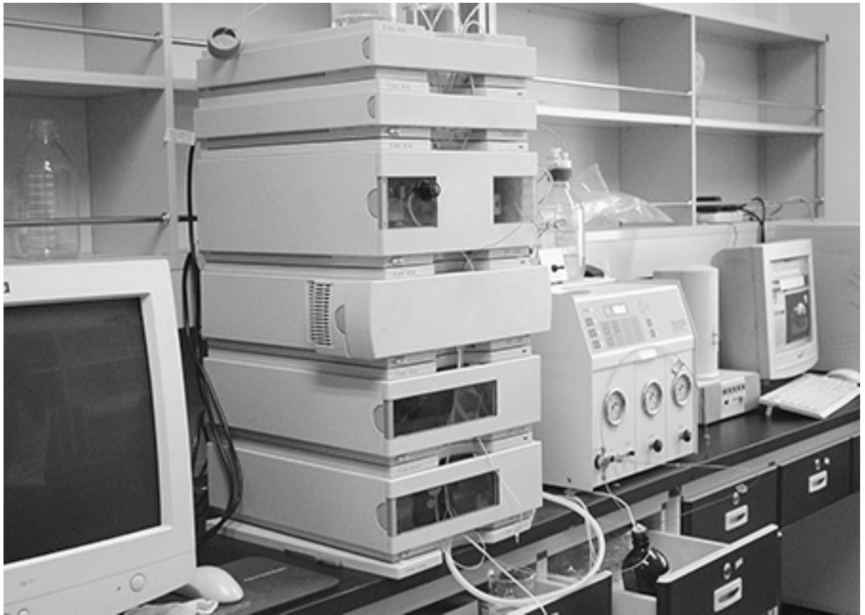
Liquid chromatographers are used for separation, identification, and quantification of high boiling point, poor heat stability, or large molecules.
