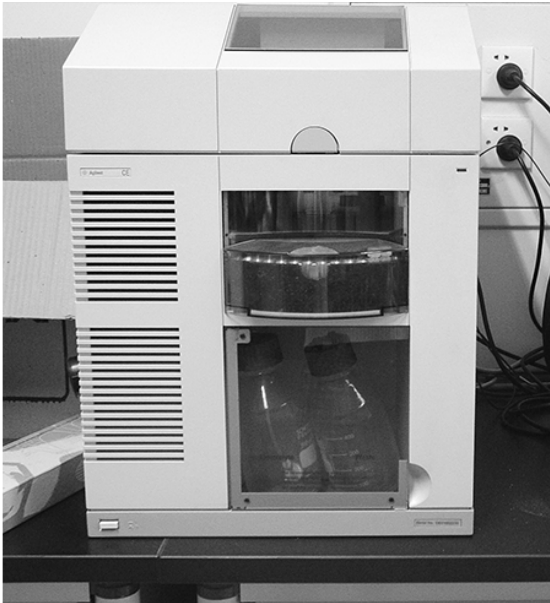
Capillary electrophoresis equipment is used to separate biopolymer, peptides and small molecules in narrow glass capillaries.
