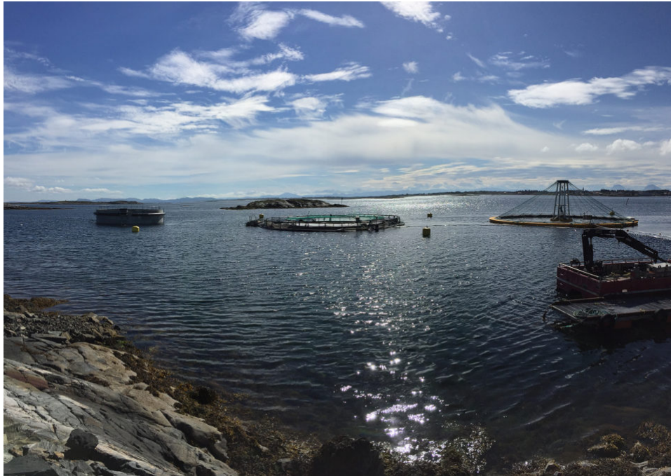
Three floating closed containment systems at Smøla/ Nekton Havbruk AS, i.e., from left to right: the "Salmon home #1" concrete tank (as it is being deployed), flexible floating semi-closed containment system, and Fiberglass AgriMarine tank. Photo by Jelena Kolarevic.
