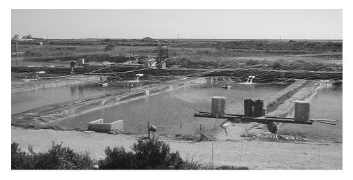
The experimental seaweed biofilter system operated at an intensive sea bream farm in southern Portugal, where flow-through fish ponds continuously supplied 12 seaweed biofilter tanks.
