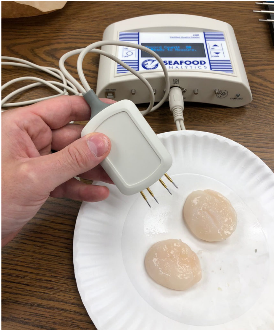
The Certified Quality Reader device has electrodes that when pressed against a specimen send an electrical signal through the animal. Photo courtesy of Seafood Analytics.
