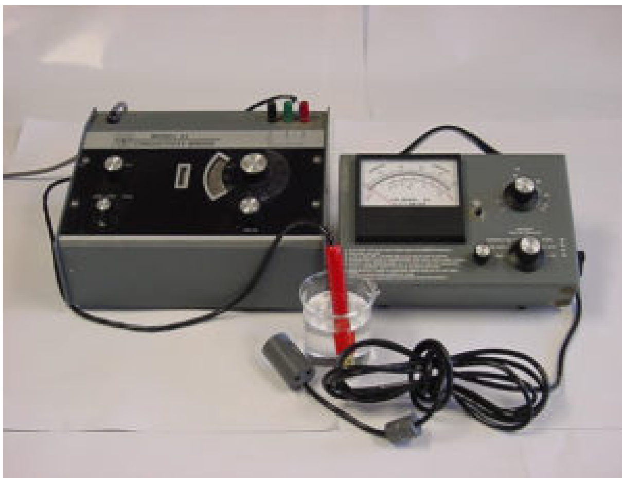
Fig. 1: A laboratory bench conductivity meter (left) and a portable conductivity meter (right).
