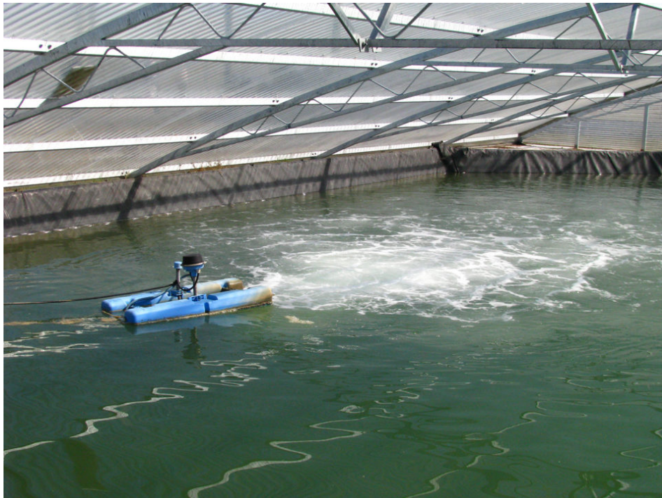
A propeller-aspirator-pump aerator.
