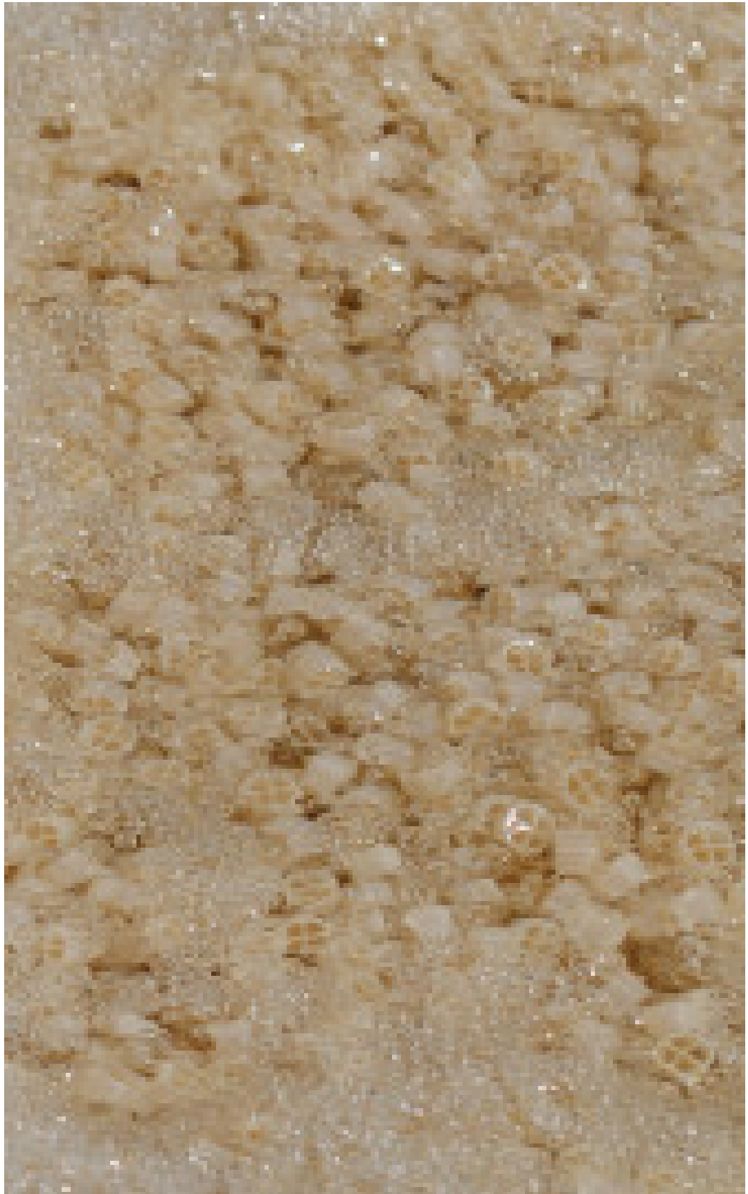
After four months, the "seasoned" media looks brownish and has less buoyancy.
