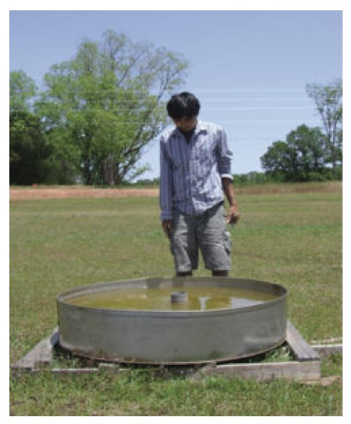
The U.S. Weather Bureau Class A evaporation pan is a common device for measuring evaporation. The amount of water lost from these pans (corrected for rainfall input) is measured daily.
