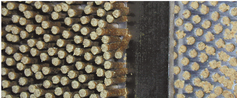
A rotating knife cuts extrudate into pellets as it emerges from the die.
