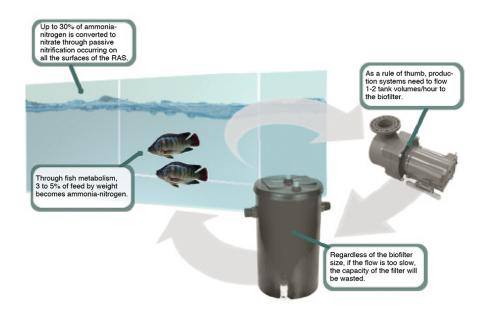
In general, an RAS requires water to flow from the culture tank to the biofilter once or twice an hour depending on the desired tank TAN concentration and biofilter efficiency.
