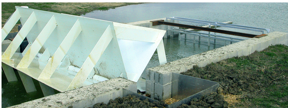
A large paddlewheel pumps water out of the fish-confinement area. Barriers prevent fish escapes.
