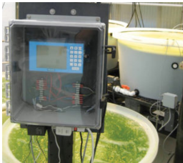
This HISTAR system controller has eight analog inputs and eight control relays.
