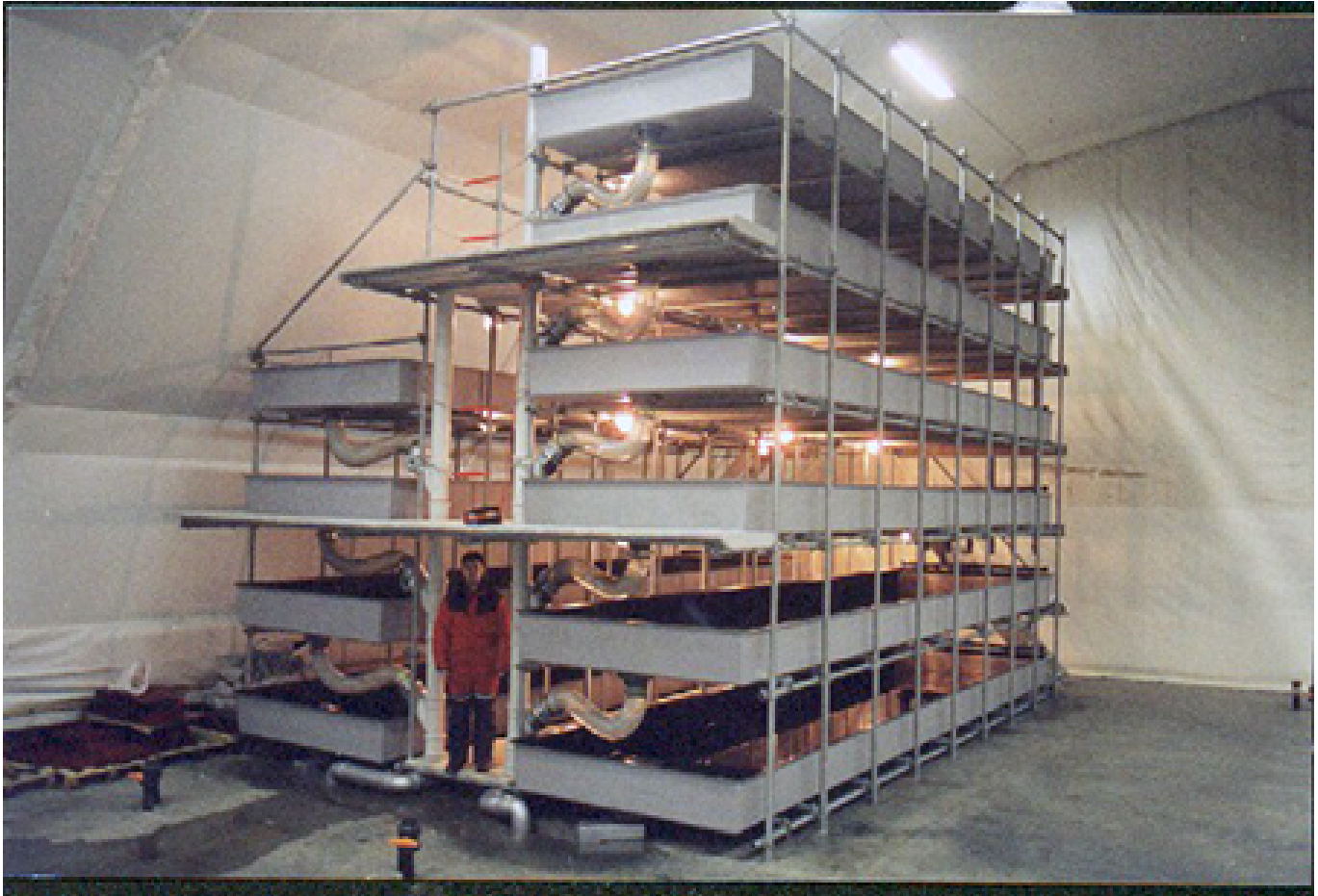
Shallow raceways can be stacked to save valuable production space. This multilevel unit is in Lofoten, Northern Norway. Photo by Dag Hansen, LOFILAB.
