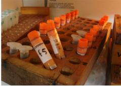
Left: View of the analytical station with titrators and central control software for pH-stat determination of protein hydrolysis at LAM-USP. Right: Ready-to-use frozen standardized enzyme extracts recovered from shrimp species for in vitro protein digestion assays at LAM-USP.
