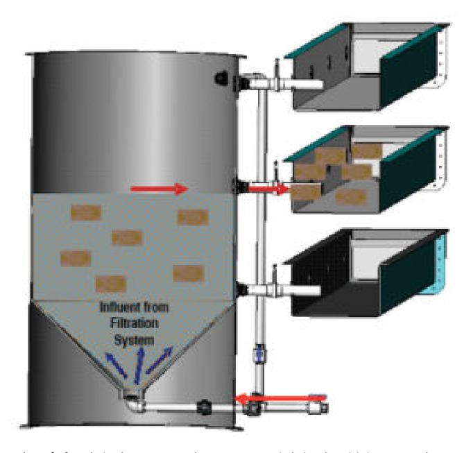
Larval transfer from the incubator system to the raceway system is designed to minimize stress on the fish.
