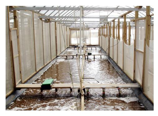
To maintain oxygen levels, the enclosed test raceways had banks of airlifts, air diffusers and Venturi injectors.
