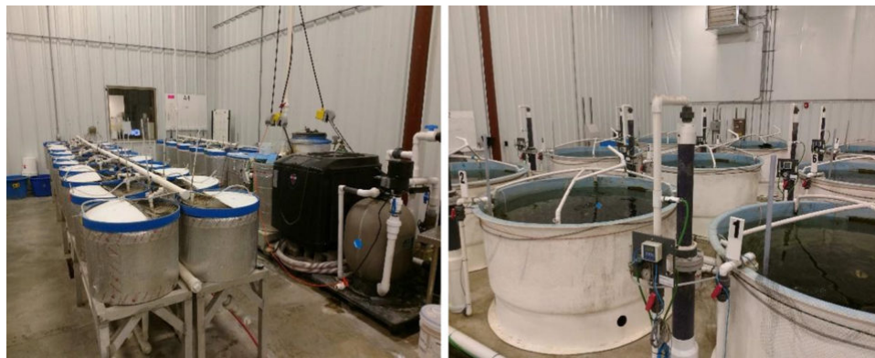
Fig. 1: Experimental recirculating aquaculture systems of the Aquatic Research Laboratory, Prairie Aquatech (Brookings, South Dakota, USA) used in the trials. The systems comprised tanks (30 × 113 liters and 8 × 757 liters) with a flow rate of 2 liters per minute, equipped with biological and mechanical filtration, UV sterilization, temperature control and pure oxygen supplementation.
