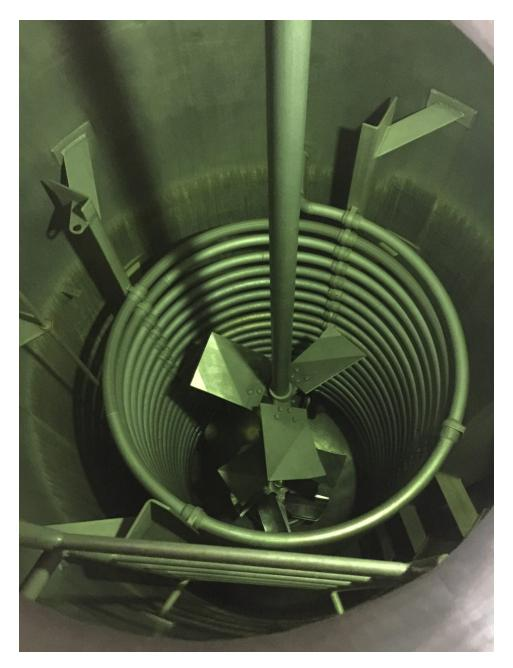
Inside a 20,000-liter fermenter used to produce KBM through the company's dedicated fermentation process. This type of equipment offers a very high degree of process control and is relatively standard equipment.
