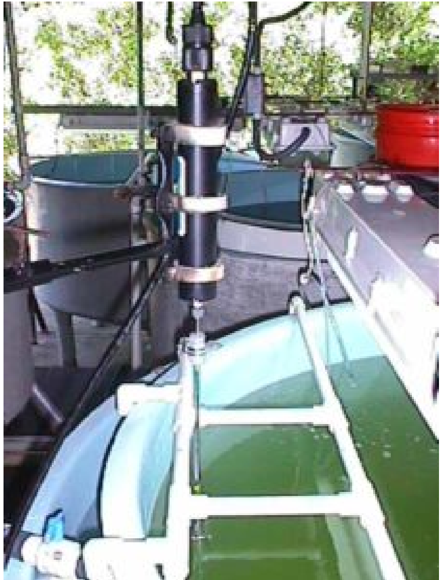
A Doppler current meter measured turbulence in the larval tanks
