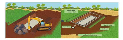
The necessary steps for the construction of a non-hazardous waste final disposal site include site selection, operation and other considerations.
