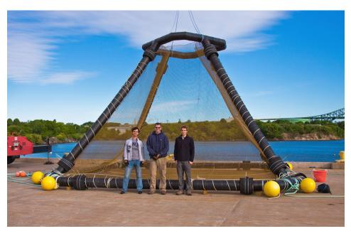
Copper alloy net cages offer increased strength and maintenance advantages, but may require special engineering for integration with existing facilities.
