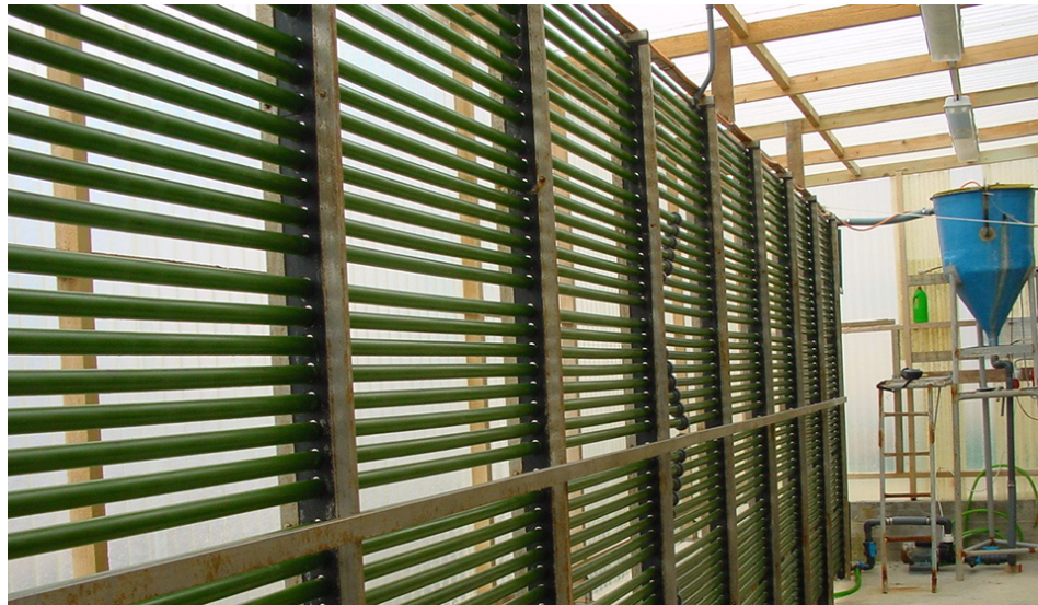
Automated, intensive algal production system.
