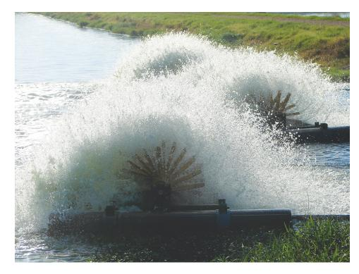
Catfish production is based largely on routine nighttime aeration with electric paddlewheel aerators.
