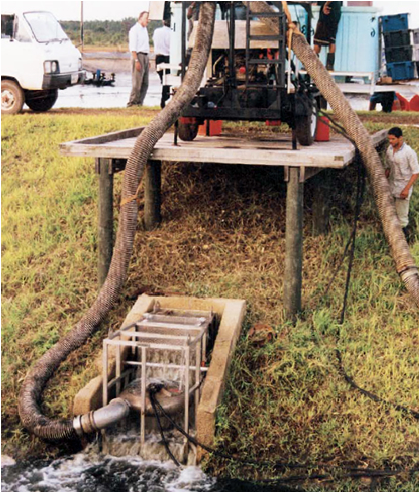
Shrimp from a draining pond (background) are lifted by recessed-impeller pump (bottom) to the de-watering tower (top) and then to ice slurry. Water from the tower drains through the hose on right to a ditch.
