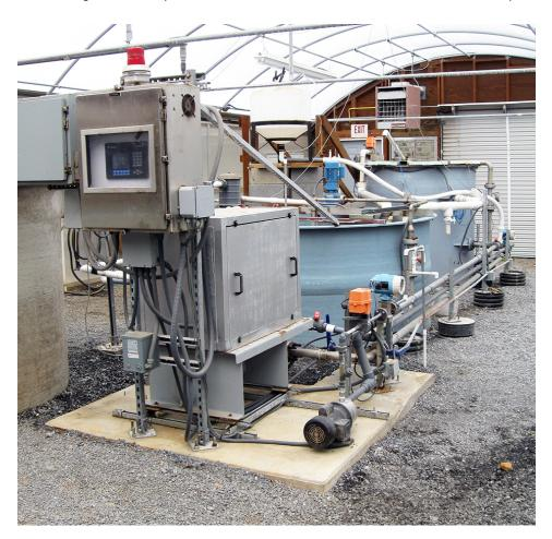
The membrane biological reactor located at the Conservation Fund's Freshwater Institute was operated for the recovery of not only water but alkalinity, salts, phosphorus and protein.
