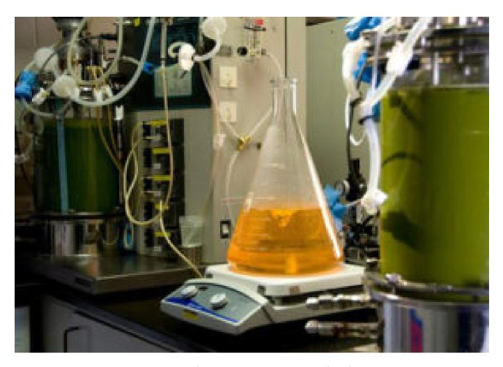
Research into the varied applications of algae is assisted by the use of 5-L fermentation vessels such as those pictured above. These vessels allow algae to be produced by a feed batch technique that results in unique nutritional properties.
