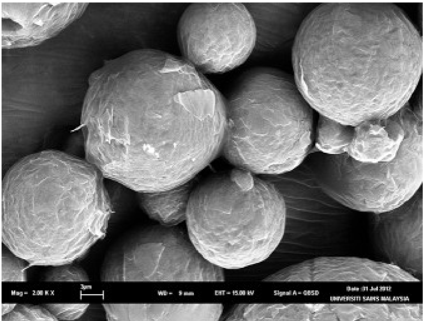
A scanning electron micrograph of the microencapsulated organic acids blend manufactured using centrifugal cool-spraying technology by Sunzen Feedtech Pte. Ltd. (Malaysia).
