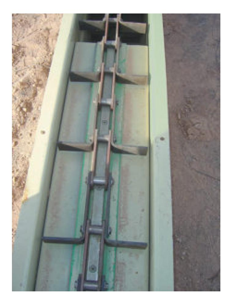
Since flushing may not remove all residues of antimicrobials from screw conveyors, drag conveyors may be more appropriate to ensure cleanliness of feed production lines.
