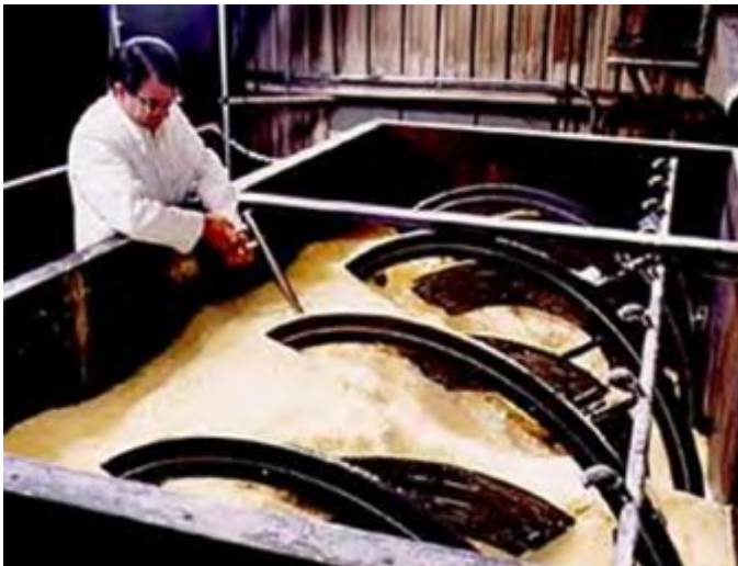
View of a horizontal, continuous ribbon mixer.
