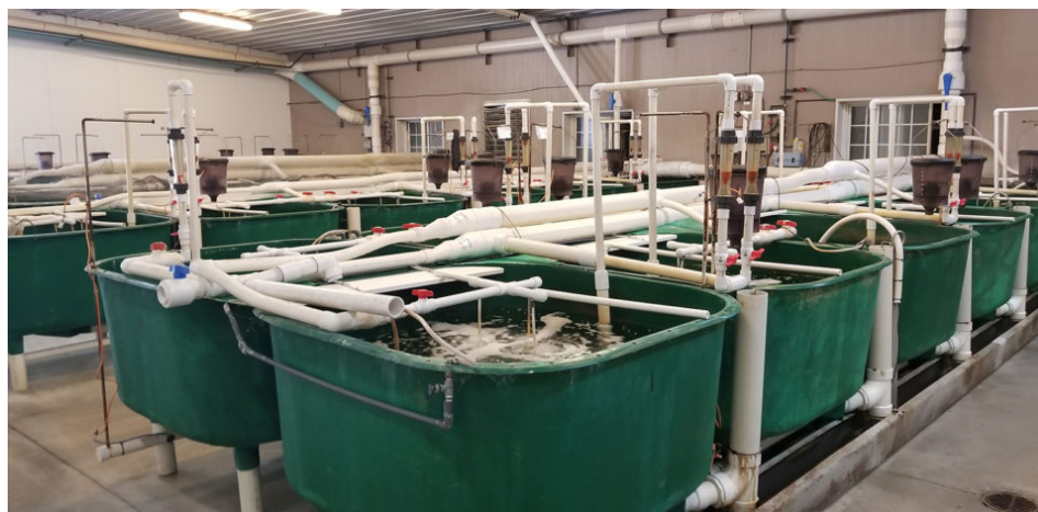
Replicated tanks linked to a RAS system where both feeding trials were completed. Photo by Tom Waldrop, Mote Marine Laboratory.
