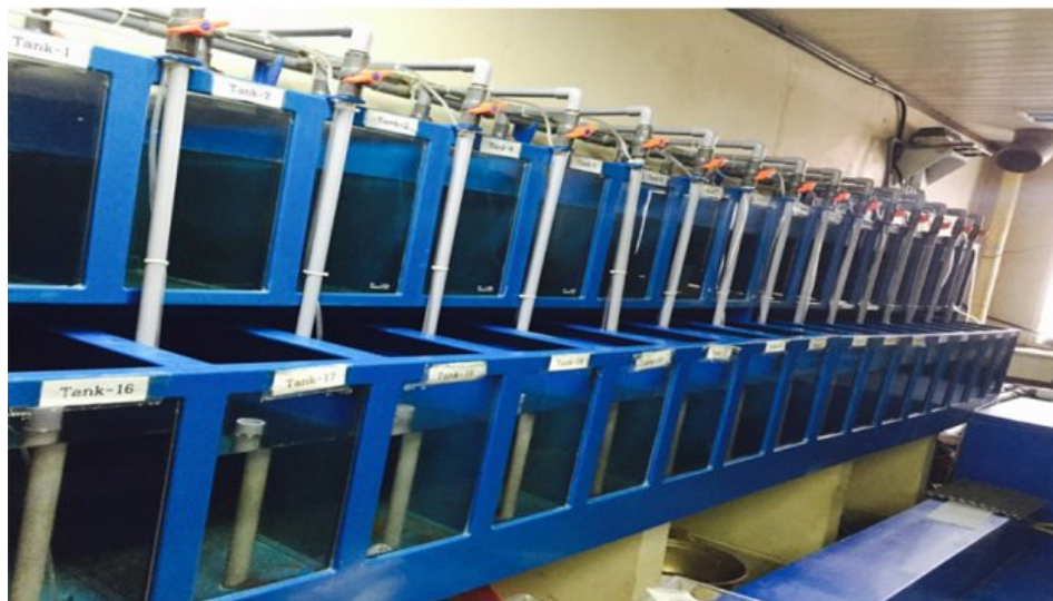
The semi-recirculation system used in the trials (FFNRC, Pukyong National University, Busan, Rep. of Korea)
