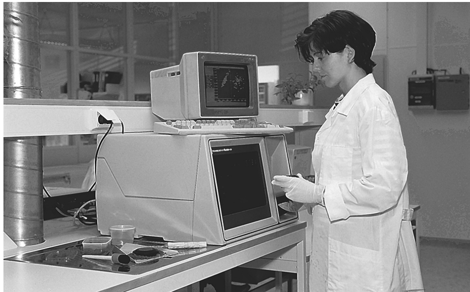
Analyzing feed composition using near-infrared reflectance.
