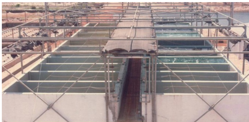
A typical shaded outdoor tank reactor phycosphere, always susceptible to eolian dust. Photo by Dr. M.R. Kitto.
