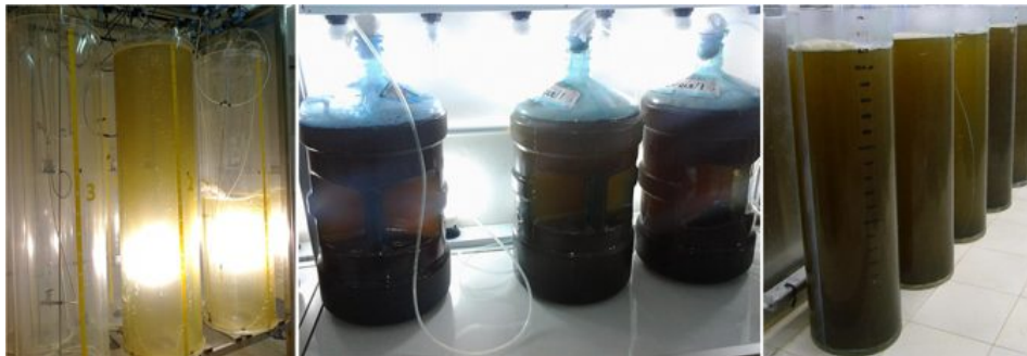
Testing growth of the diatom Thalassiosira weissflogii in containers with walls of different thickness, including 30 mm (left), 210 mm (center) and 450 mm (right).
