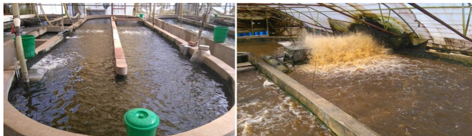
Chambo Fisheries nursery tank close-up (left); Front view of 10-Hp paddlewheel aerator at Chambo Fisheries (right).
